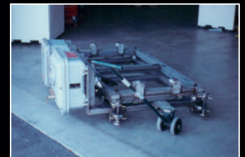
Portable rocket fuel scale, 50,000-lbs x 1.0-lb increments with explosion proof NEMA7/9 enclosure
